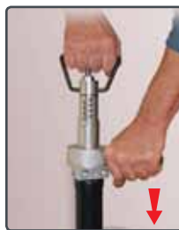
Extract the stem puller and lock it with a light rotation towards right or left..
