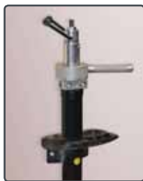
Screw the stem puller in the support by positioning the unit on the shock absorber and fix the stem of the cylinder with the locking nut
