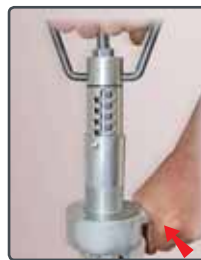
In case the buffer has not come out completely after this first step, it is possible to extract the stem by another 20 mm by keeping the handle still and rotating the stem puller.
