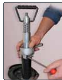
When the extraction is complete, lock the clamp with the appropriate screws.
