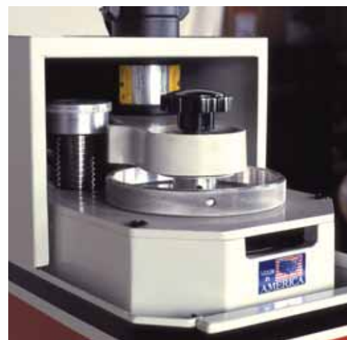
Quick cutterhead change draw bar system
